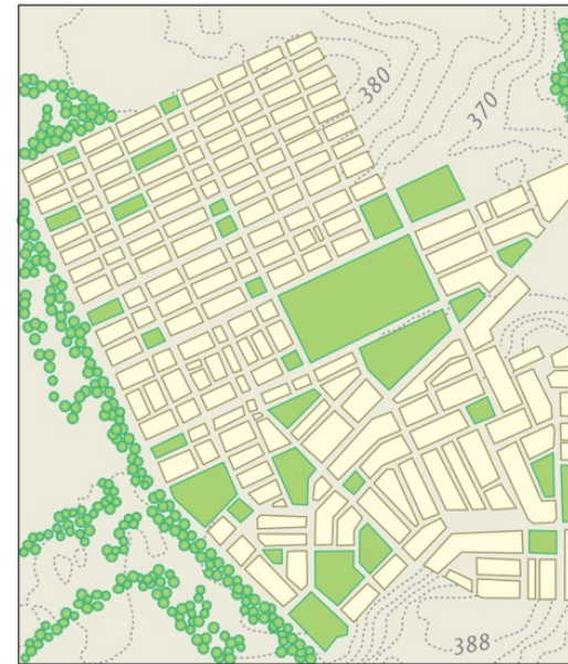
Figure 15.5 Alternative layout plans for the Koufan extension zone in Tahoua, Republic of Niger. The official plan (a) is based on a generic grid design (b) an alternative plan based on local climate and topography. (Oke et al. 2017)
